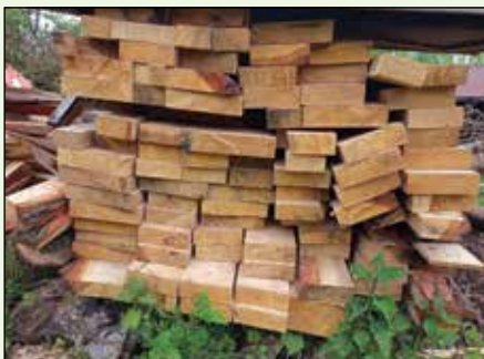
Local oak planks drying
